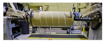
Fully Distributed Regulating Voltage Winding
